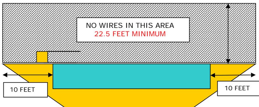
No overhead wiring shall be installed within **22.5 feet (6.9 m)** vertically from the water and all areas extending **10 feet (3.05 m)** horizontally from the inside of the walls of the pool. Wiring above diving structures, observation stands, towers, or platforms shall not be within **14.5 feet (4.40 m)**.
